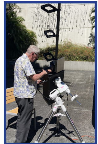
Dr. Adalbert Ding calibrating the lab instrument for outdoor testing of the occulter and tripod sun tracker.
