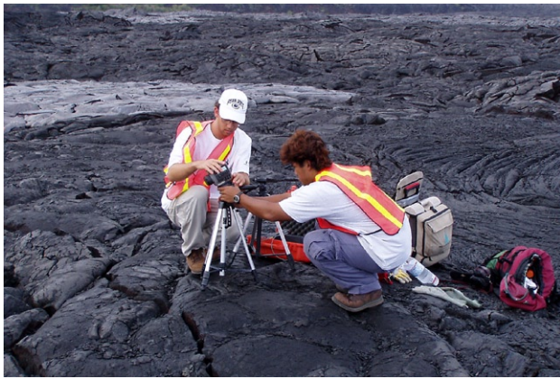
Graduate students LEON GESCHWIND and STEVE SAHETAPY-ENGEL perform temperature measurements to determine cooling rates of active lava flows. These data are then compared with remote sensing observations from NASA's Landsat 7, Hyperion, and MODIS instruments.
