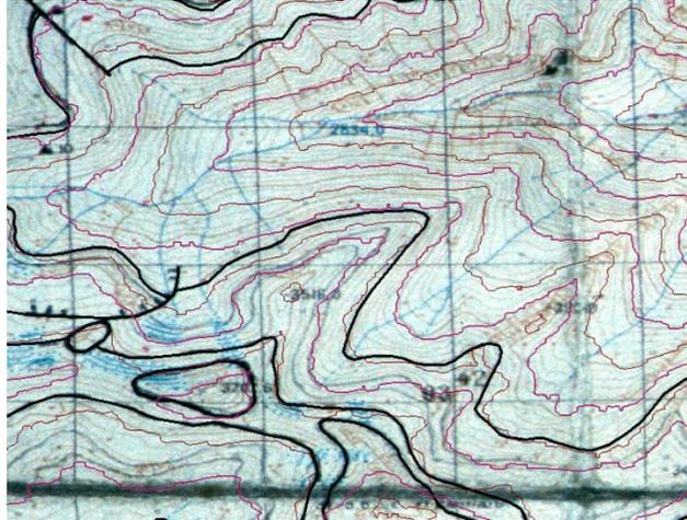
*Figure 2: The high degree of agreement between the ASTER derived contour lines and the topographic map contours assured the georectification of the base maps was accurate. NASA ASTER Program (2011).*
