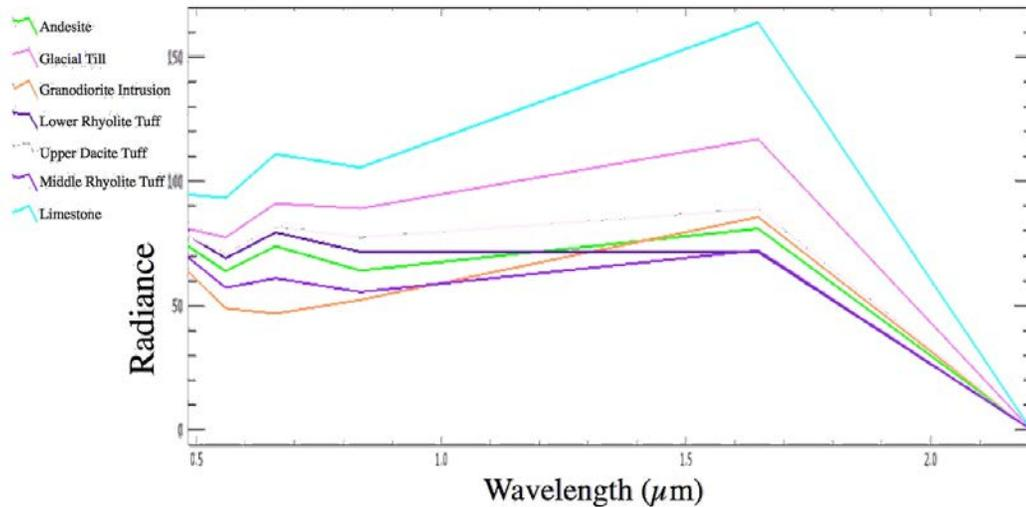
Figure 3: Spectral signatures of the limestone and igneous geologic units. NASA Landsat Program (1999).
