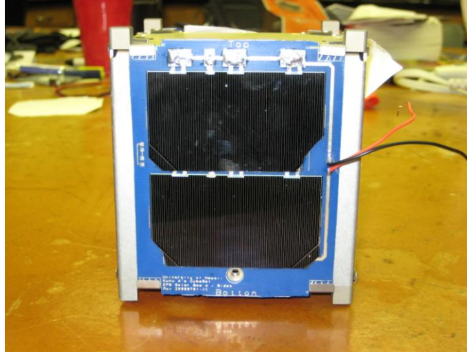
Figure 2: Populated Solar Panel on Engineering Model (EM)
