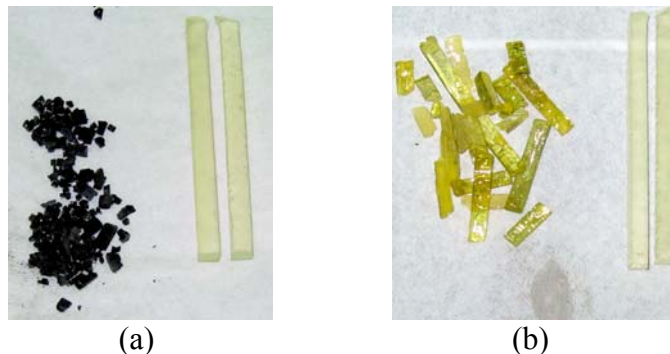
Figure 1. (a) Pyrolysis of pure ceramic at 1100°C, (b) Pyrolysis of pure ceramic at 550°C
