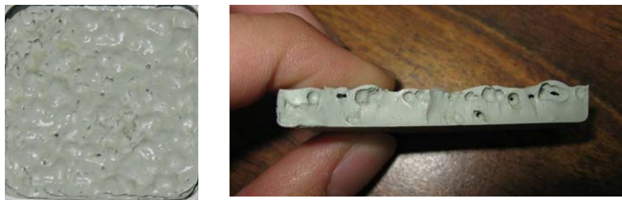
Figure 4. Pictures of a sample with 15 wt% nanoparticles and 40% solvent. Left: Top view of the sample. Right: Side view of the sample cross-section.
