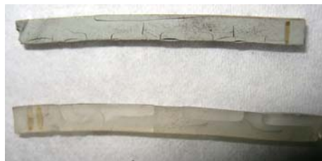
Figure 2. Samples pyrolyzed at 450°C, top sample contains 2.5 wt% nanoparticles & bottom sample is from pure polymer.
