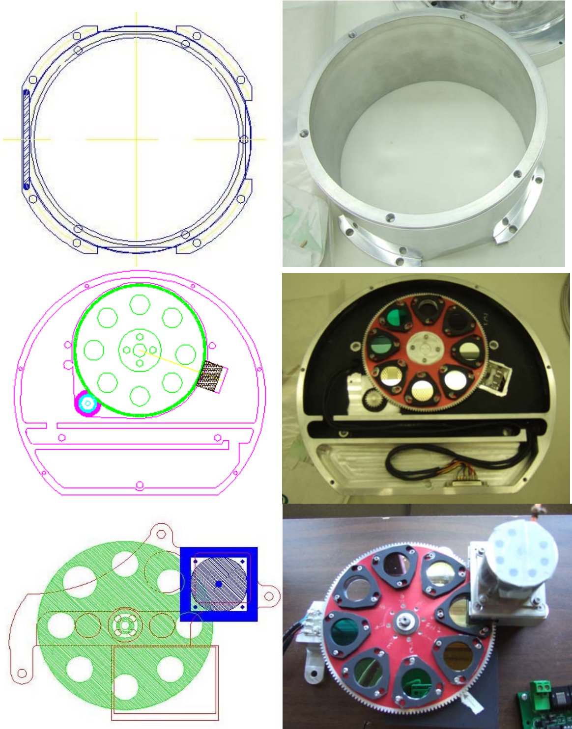
Figure 1: AutoCAD drawings for three components of QUIRC; 'Shield 1' (top), Filter Wheel Assembly I (middle), Filter Wheel Assembly II (bottom).
