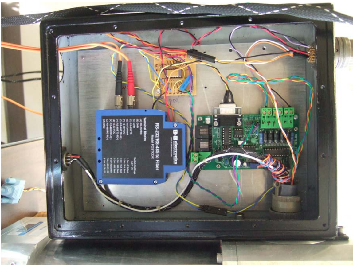
Figure 2: The QUIRC Electronics 'black box' that now houses the electronics to control the filter wheel. The hardware includes a Hall-Effect Amplifier circuit board (top), Pontech STP Stepper Motor Controller (bottom right) and B&B Electronics RS 232 to Fiber Optic Converter.
