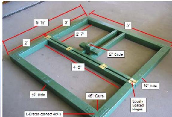
Figure 2: Square bottom of antenna base
