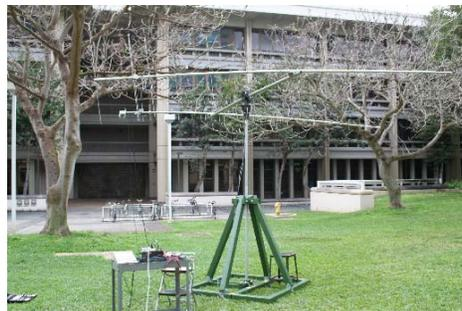
Figure 5: Complete raised VHF/UHF mobile-modular ground station
